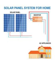
Most, if not all, appliances in you home run on either 110 or 240 Alternating Current (AC). We therefor need to convert the DC into AC and that is what we need the inverter for. The inverter converts DC to AC and works as an interface between the solar panels and your AC electric system of your house and the grid.
