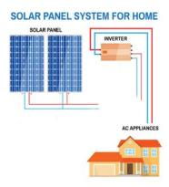
Most, if not all, appliances in you home run on either 110 or 240 Alternating Current (AC). We therefor need to convert the DC into AC and that is where we need the Inverter for. The inverter converts DC to AC and works as an interface between the solar panels and your AC electric system of your house and the grid.
