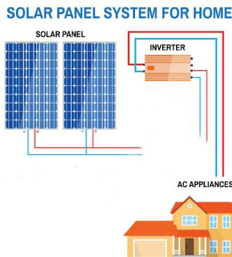
Most, if not all, appliances in your home run on either 110 or 240 Alternating Current (AC). We therefore need to convert the DC into AC and that is where we need the Inverter for. The inverter converts DC to AC and works as an interface between the solar panels and your AC electric system of your house and the grid.
